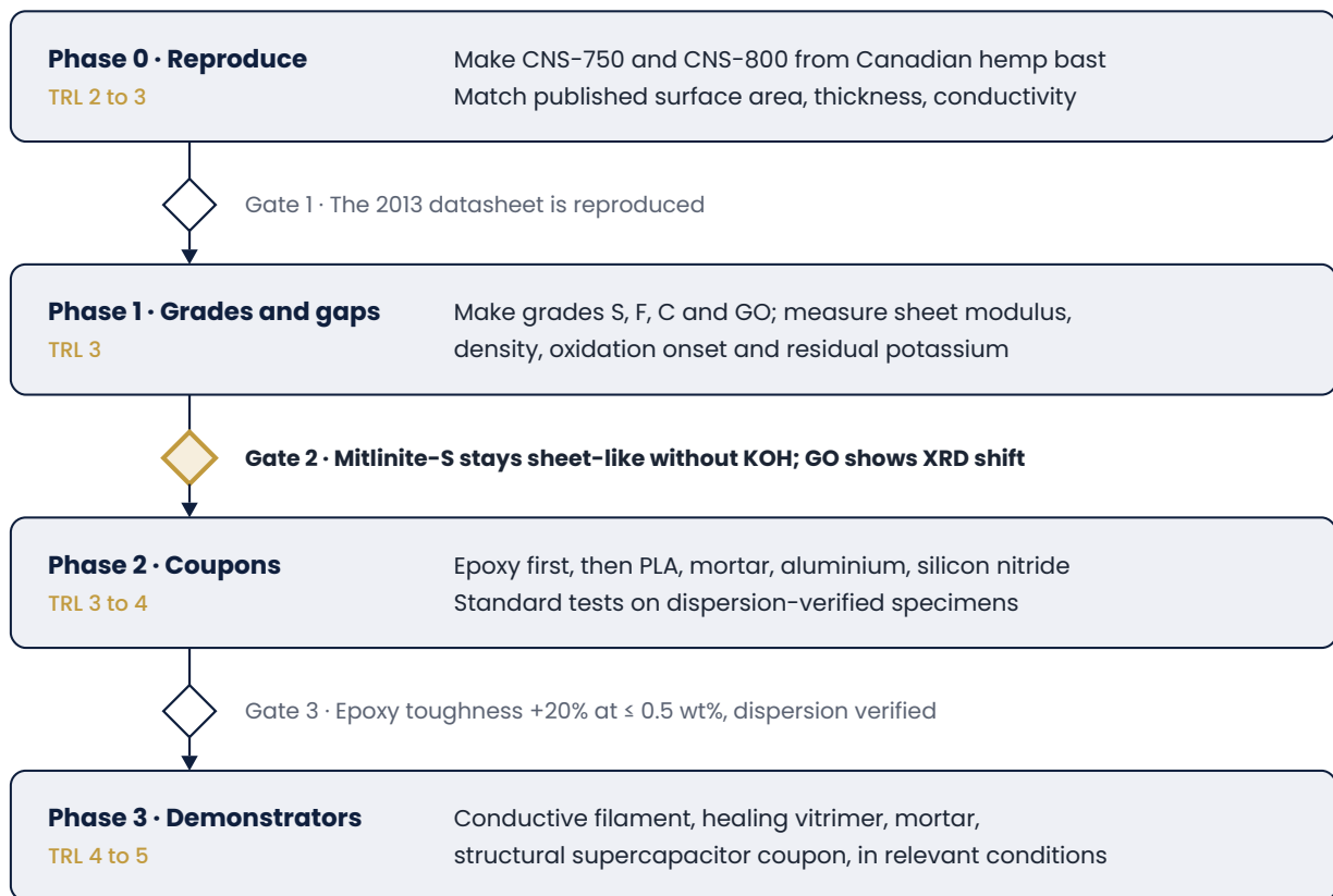
Figure 12.1 Four gated phases take Mitlinitite composites from TRL 2 to TRL 5. A phase starts only when the gate above it is passed; the highlighted gate is decisive. No dates are set.
