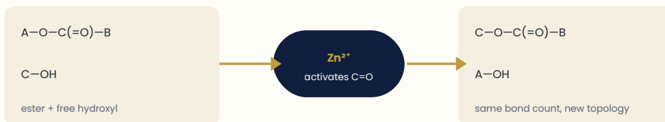
FIGURE 3 · Cure and exchange chemistry. The acid-epoxy reaction creates \beta -hydroxy esters; \text{Zn}^{2+} catalyses their associative exchange, the mechanism Leibler's group introduced for epoxy vitrimers [4].
